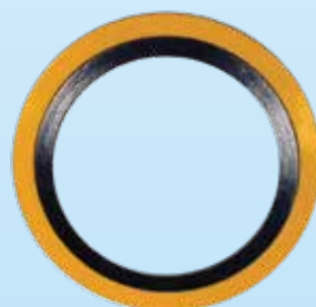
CG TYPE SPIRAL WOUND GASKET OUTER RING : CARBON STEEL HOOP: SS304 FILLER: GRAPHITE CLASS 150, 300 & 600 ASTM B16.20
