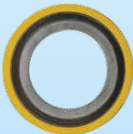
SPIRAL WOUND GASKET w/ CENTER RING OUTER RING : CARBON STEEL HOOP: SS304 FILLER: GRAPHITE CLASS 150, 300 & 600 ASTM B16.20
