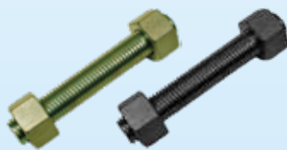
STUD : ALLOY STEEL NUTS: CARBON STEEL ASTM A-193 GRADE B7 FOR STUDS ASTM A-194 GRADE 2H FOR NUTS
